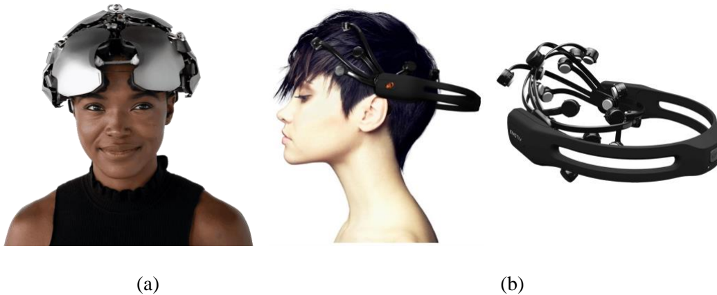
Fig. 2. Examples of non-invasive BCIs by Kernel and Emotiv. The ‘Kernel Flow’, this is a non-invasive BCI, that can be used for recording real time cortical hemodynamics to establish precise patterns of brain activity (a). The aim of the company is to ‘make measurements of the brain and mind mainstream’. Another example of non-invasive BCI: EMOTIV EPOC, a type of non-invasive BCI, which allows users to gain an accurate insight into their cognitive and emotional state in real-time by means of electroencephalography (EEG). EMOTIV’s analyses can be used to improve your performance and develop new applications and services in neuroscience research, health and wellness, automotive, consumer research, education and entertainment (b).
